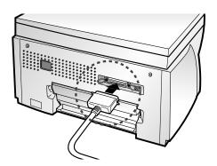
**3** Push the metal clips down to fit inside the notches on the cable plug.
